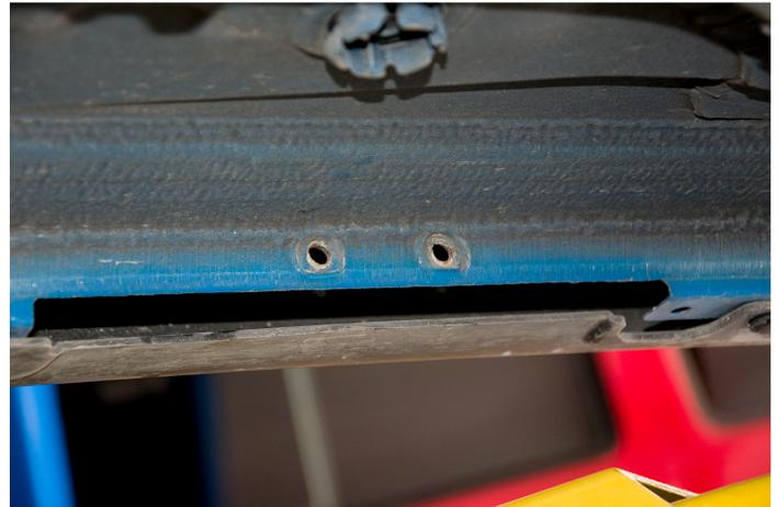
With the holes drilled get your 5/16-18 hex head bolt with jam nut and 2 zinc thrust washers as well as the 12 – Aluminum Nut-serts.
