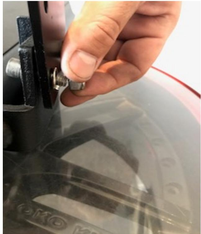
After installing the three brackets to the first side step repeat the process for the second step. Tighten down the bolts/nuts so that the tops of the angle bracket sit level in reference to the length of the side step. They should now both look like this.
