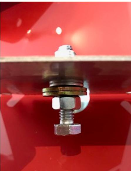
Tighten the jam nut using the open end of the wrench while holding pressure with the socket preventing the bolt from turning in the Nut-Sert. Doing this will collapse the Nut-Sert. Repeat this on the remaining holes.
