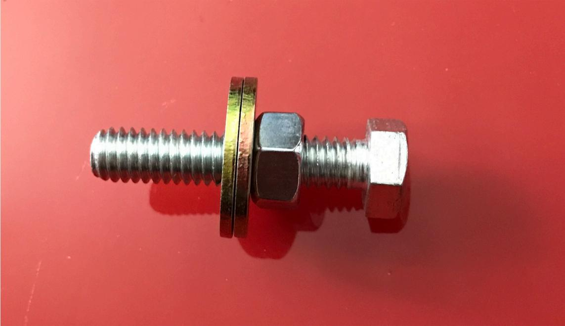
Coat the threads of the 5/16 bolt with anti-seize and thread 1 Aluminum Nut-Set onto the bolt making sure that you have full thread penetration on the nut set.
