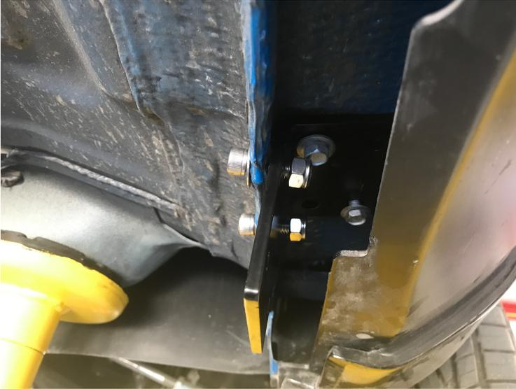
Take the remaining 12 – 5/16 Allen Bolts and secure the bracket to the pinch weld using the lock washer and the nylock nut.
