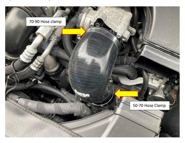
10. Re fit the rubber air intake hose and that is the installation complete. Follow these steps in the same order for the other throttle body. Once completed take your vehicle for a test drive and enjoy your new Forge Motorsport product.
