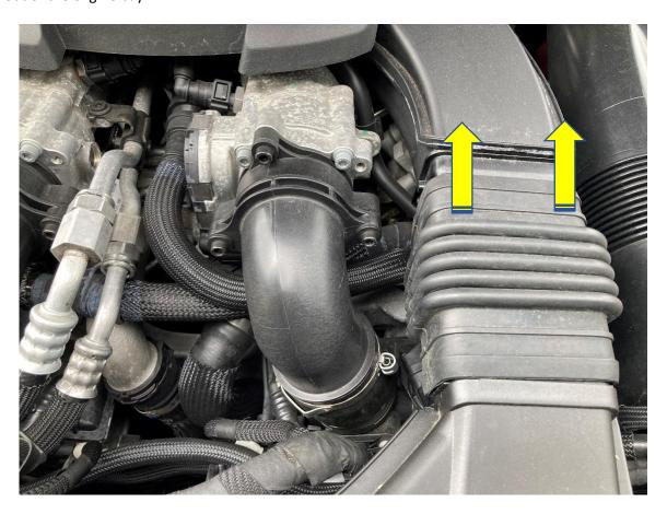
2. Remove X2 M6 fasteners, use a 5mm Allen key to do this.
