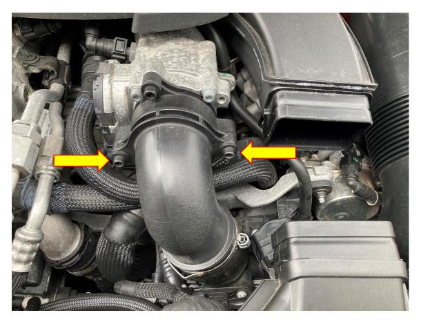
3. Undo the hose clamp attaching the throttle body hose to the charge cooler, use a 7mm socket and rachet or hose clamp removal tool to do this.
