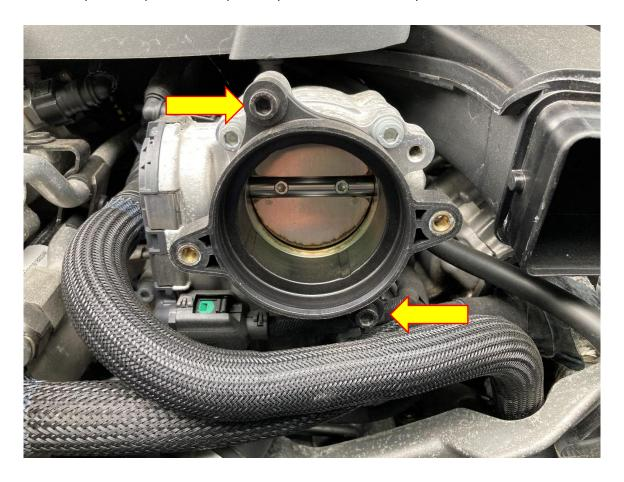
6. Remove the original rubber O-ring from the throttle body adaptor, be careful not to damage the O-ring.
