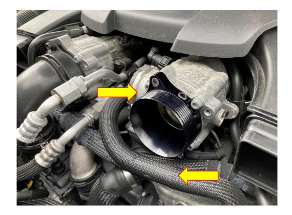
9. Fit the Forge silicone hose to the charge cooler first then to the throttle body. Use the supplied hose clamps to attach the hose, The 50-70mm hose clamp for the charge cooler side of the hose and the 70-90mm hose clamp for the throttle body side.
