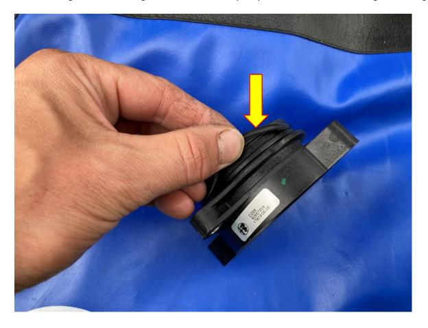
7. Fit the O-ring removed from the previous step to the machined billet adaptor from the Forge FMTBINL1 kit.
