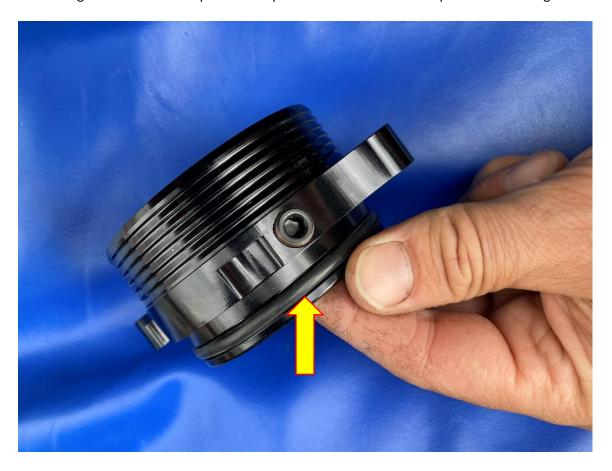
8. Fit the FMTBINL adaptor to the throttle body, use the supplied M6 fasteners and a 5mm Allen key to attach it.
