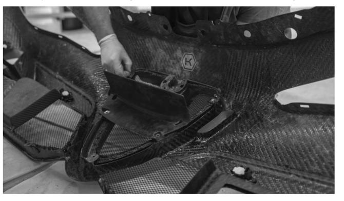
After cut is made on the mesh, install two caps using glue in small portions of dots like shown on the image below
