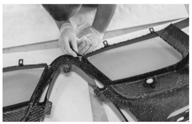
Position Front Bumper on car with Sensor Frame included on the kit make marks for the cut and cut it with Dremel or diamond disk tooling.
