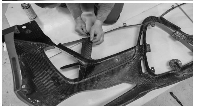
After positioning Flaps, continue with Sensors as shown below, use structural glue to attach heads.
