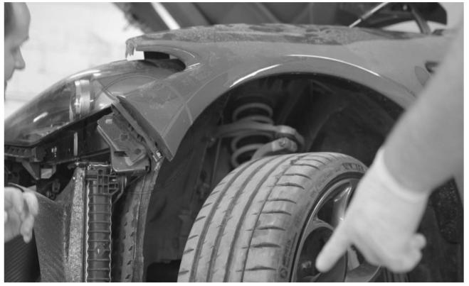
Position the Front Bumper and tighten every screw including those of Aero Front Splitter, use glue to attach the second (aesthetic) Front Parking Sensor Frame.
