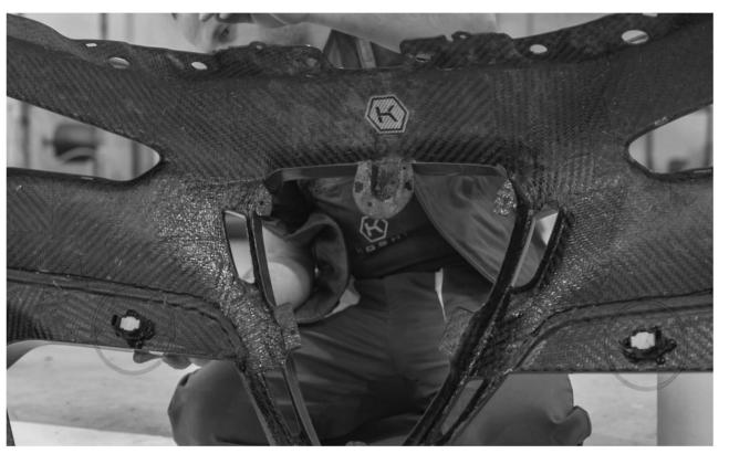
Curve mesh edges to match shape of Bumper frame, apply glue in small seamless portions.
