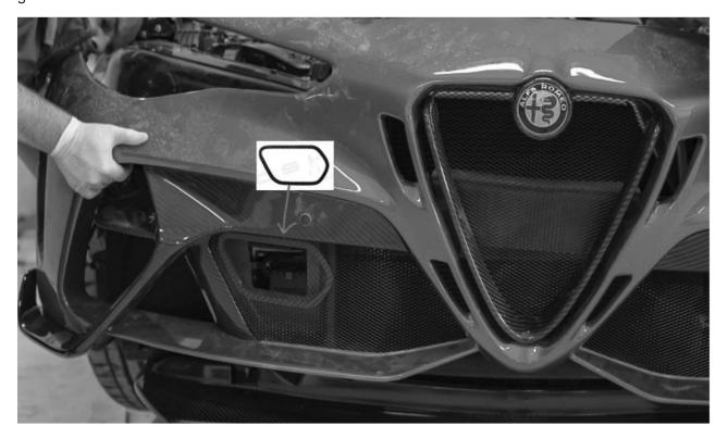
Replace Splay Intercooler Air Intake, use mesh from OEM Intercooler Frame
