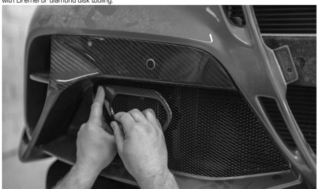
After cutting there is another Sensor Frame which fits behind aesthetic sensor frame which should be glued over the mesh.
