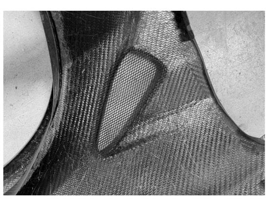
Second install the Carbon Fiber frame on top of the Side Fender mesh like shown below
