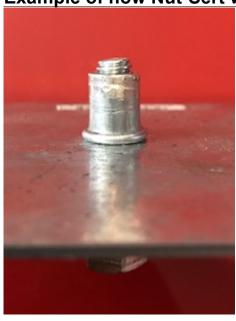
With all of the holes fitted with the Nut-Serts loosely bolt the mounting brackets back to the side steps.
