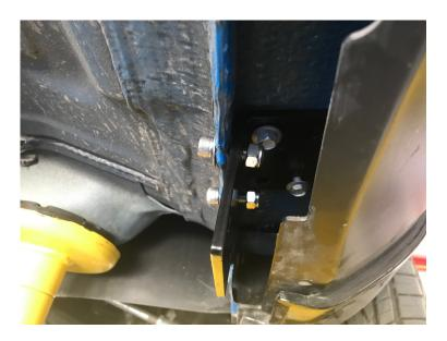
Take the remaining 12 - 5/16 Allen Bolts and secure the bracket to the pinch weld using the lock washer and the nylock nut.
