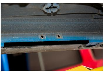
With the holes drilled get your 5/16-18 hex head bolt with jam nut and 2 zinc thrust washers as well at the 12 - Aluminum Nut-serts.
