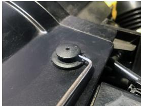
3. Remove the 5 torx bolts (T30) that run along the bottom side (underneath) of the bumper cover.
