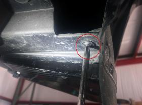
5. Using a nylon pry tool gently pry along the front of the fender flare to release it from the front bumper. Underneath there are 2 small hex bolts that you need to remove. Do this on both sides.
